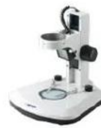
SL1 Arm stand base with fixed focus holder and LED Illumination
